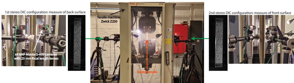
Figure 2 Illustration of the DIC experimental setup: 2 stereo configurations were used simultaneously
